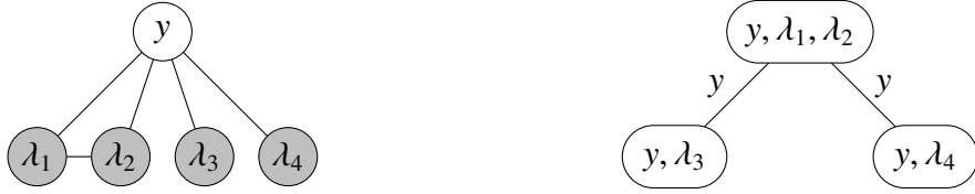
Figure 5.3: An example of a labeling function dependency graph G_\lambda (left) and its junction tree representation (right), where y is a vector-valued random variable with a feasible set of values, y \in \mathcal{Y} . Here, the output of labeling functions 1 and 2 are modeled as dependent conditioned on y . This results in a junction tree with singleton separator sets, y . Here, the observable cliques are O = \{\lambda_1, \lambda_2, \lambda_3, \lambda_4, \{\lambda_1, \lambda_2\}\} \subset \mathcal{C} .
